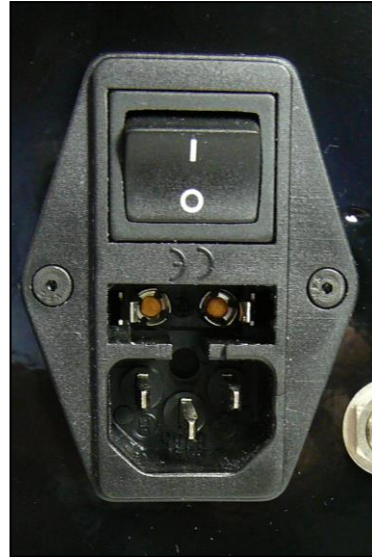
FUSE HOLDER REMOVED
